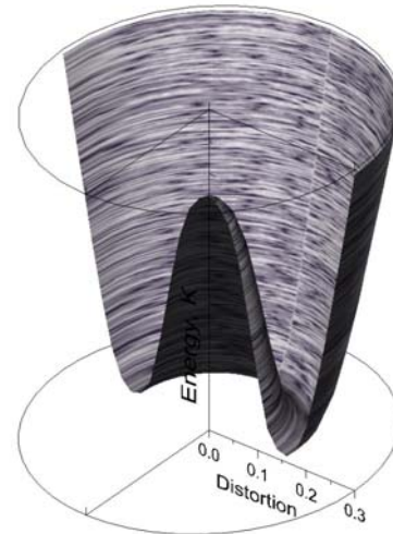
Fig. 2 Total energy vs. distortion for one of the soft phonon modes in \epsilon -Pu which reveals a double well behavior and highlights the importance of anharmonic effects. After [2].
